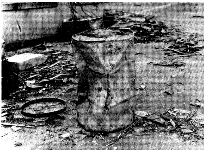
FIGURE 31 (above). A 46-gal empty 16 B.S.W. drum with central filler cap missing collapsed by the blast at Hiroshima.
